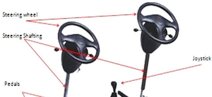
Figure 17. Preparation of 2 Assemblies of Steering Wheel
