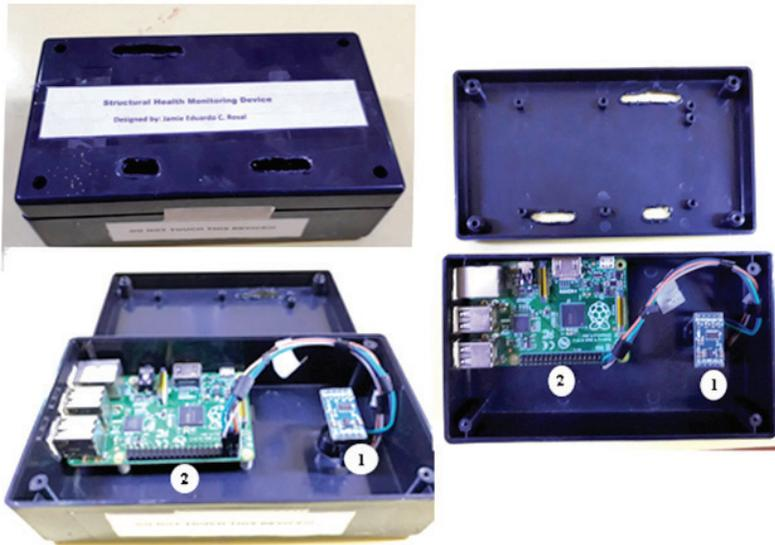
Fig. 4. Final prototype. Accelerometer sensor (1), Raspberry Pi 3 (2)
