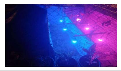
Note: The figure displays the experimental setup of blue and purple LED arrays positioned 50 cm above the plots, controlled by an automated LDR-based
