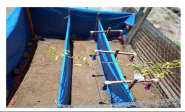
Note: The figure shows the LED lighting system integrated with LDR sensors, enabling automatic activation of blue and purple lights during low-
