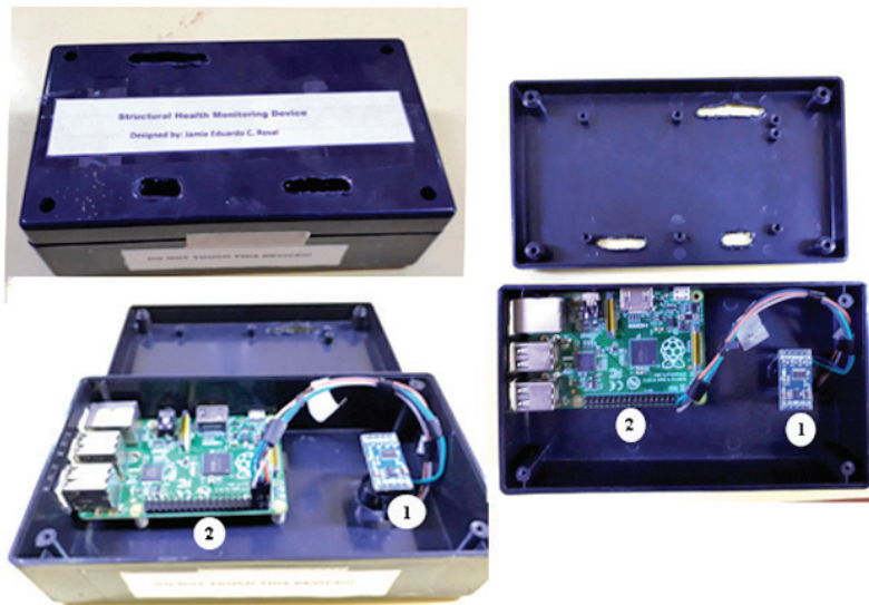
Fig. 4. Final prototype. Accelerometer sensor (1), Raspberry Pi 3 (2)
